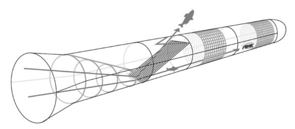
Schematic illustration of a size and species selective trawl. Entering fish are led towards the trawl floor and grid via a leading funnel. Larger fish are then led out of the trawl by the grid while smaller fish and Norway lobster pass through the grid and enter the codend. The full square mesh codend enhances escapement of small fish and undersized Norway lobster. The square mesh codend shown in the diagram is required only in Skagerrak and Kattegat.
