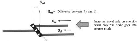
Compensator geometry allows equal tension in both rear cables
