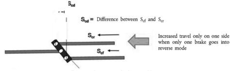
Compensator geometry allows equal tension in both rear cables
