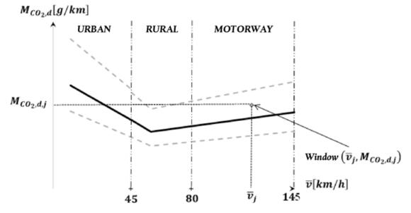
*Figure 6* Vehicle CO<sub>2</sub> characteristic curve: urban, rural and motorway driving definitions (Illustrated for OVC-HEV vehicles) except N2 category vehicles that are equipped in accordance with Directive 92/6/EEC with a device limiting vehicle speed to 90 km/h)
