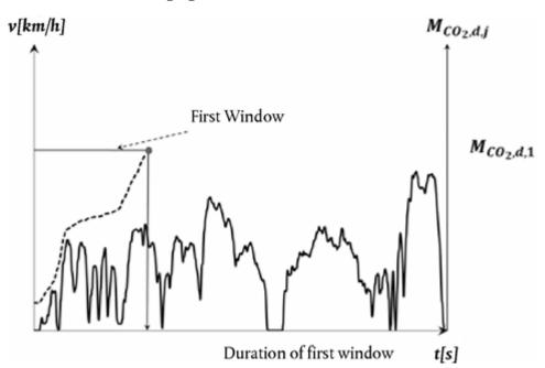
Figure 2 Definition of CO<sub>2</sub> mass based averaging windows
