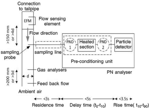
The PN analyser shall be connected to the sampling point via a sampling probe which extracts a sample from the centreline of the tailpipe tube. As specified in point 3.5 of Appendix 1, if particles are not diluted at the tailpipe, the sampling line shall be heated to a minimum temperature of 373 K (100 °C) until the point of first dilution of the PN analyser or the particle detector of the analyser. The residence time in the sampling line shall be less than 3 s.
