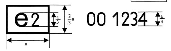
The above approval mark affixed to a component of a replacement pollution control device shows that the type concerned has been approved in France (e 2), pursuant to this Regulation. The first two digits of the approval number (00) indicate that this part was approved according to this Regulation. The following four digits (1234) are those allocated by the approval authority to the replacement pollution control device as the base approval number.
