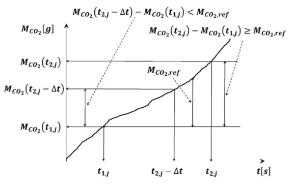
The duration  $(t_{2,j} - t_{1,j})$  of the j<sup>th</sup> averaging window is determined by:  $M_{CO_2}(t_{2,j}) - M_{CO_2}(t_{1,j}) \ge M_{CO_2, ref}$
