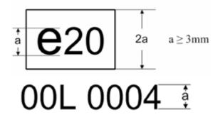
The above certification mark affixed to an axle shows that the type concerned has been approved in Poland (e20), pursuant to this Regulation. The first two digits (00) are indicating the sequence number assigned to the latest technical amendment to this Regulation. The following letter indicates that the certificate was granted for an axle (L). The last four digits (0004) are those allocated by the type-approval authority to the axle as the base certification number.
