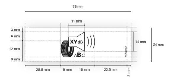
2.1.2. Format of the bottom part of the tyre label for tyres which satisfy the minimum snow grip index values set out in UNECE Regulation No 117:
