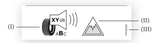
1.5. Information to be included in the bottom part of the tyre label for tyres which satisfy both the relevant minimum snow grip index values set out in UNECE Regulation No 117 and the minimum ice grip index values:
