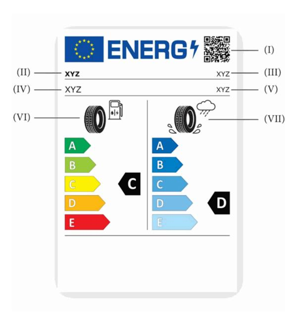
1.2. Information to be included in the bottom part of the tyre label for all tyres other than tyres which satisfy the minimum snow grip index values set out in UNECE Regulation No 117, or the relevant minimum ice grip index values, or both:
