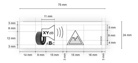
2.1.4. Format of the bottom part of the tyre label for tyres which satisfy both the relevant minimum snow grip index values set out in UNECE Regulation No 117 and the minimum ice grip index values:
