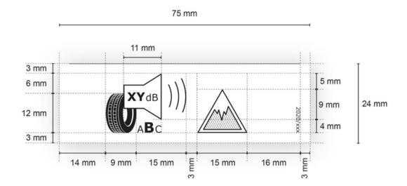
2.1.4. Format of the bottom part of the tyre label for tyres which satisfy both the relevant minimum snow grip index values set out in UNECE Regulation No 117 and the minimum ice grip index values:
