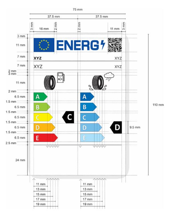
2.1.1. Format of the bottom part of the tyre label for all tyres other than tyres which satisfy the minimum snow grip index values set out in UNECE Regulation No 117, or the relevant minimum ice grip index values, or both:
