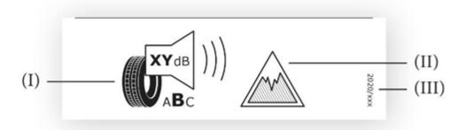
1.5. Information to be included in the bottom part of the tyre label for tyres which satisfy both the relevant minimum snow grip index values set out in UNECE Regulation No 117 and the minimum ice grip index values:
