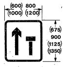
Right hand lane of a two lane carriageway of a dual carriageway road closed to traffic ahead
