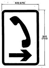
Direction to an emergency telephone or to a telephone at or near a level crossing 855
