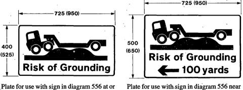
Plate for use with sign in diagram 556 at or near a railway level crossing or with sign in diagram 528 at or near a hump bridge 556.1 Plate for use with sign in diagram 556 near a railway level crossing or with sign in diagram 528 near a hump bridge 556.2 (8) Deleting diagrams 564.2, 564.3 and 564.4 in Schedule 1 Part II.
