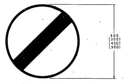
End of maximum speed limit indicated by diagram 670 671
