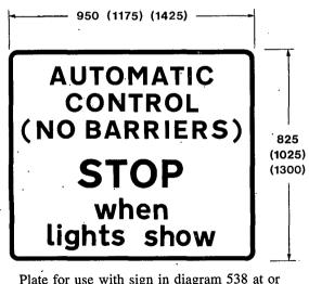
Plate for use with sign in diagram 538 at or near a level crossing where signals prescribed by Regulation 13(4) are installed 537.4
