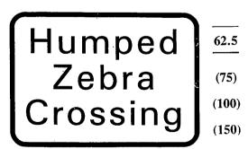
Plate for use with sign in diagram 544 in cases where a road hump is co-incident with the black and white striped area of a zebra crossing.
