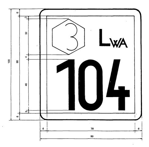
All the dimensions shown above may be multiplied, for example by  $\frac{1}{2}$ ,  $\frac{1}{3}$ , 2, 3, 4 etc., and a tolerance of 20% shall be allowed on all the dimensions.
