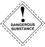
Packages containing two or more dangerous substances which have different characteristic properties. Mixed hazards.
