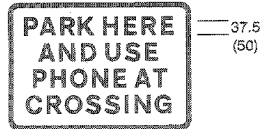
786 Place where large or slow vehicles should wait near an automatic railway or tramway level crossing while the driver obtains permission to cross
