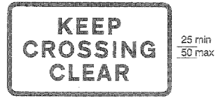
775 Vehicular traffic must not stop within the area of a railway or tramway level crossing
