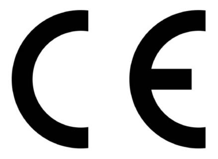
The marking may be reduced or enlarged but the proportions given in the above drawing must be respected.
